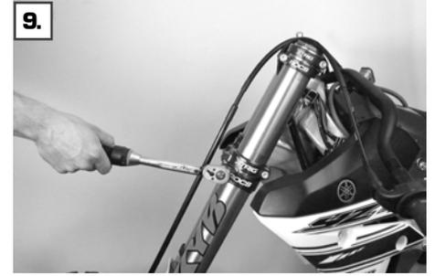
Tighten the bolts M8x40 (9) of the lower triple clamp to 15 Nm. Reinstall the front fender and brake line guide
