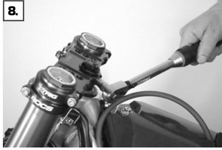
Tighten the bolt M8x25 (8) to clamp the shaft tube with 20 Nm.
