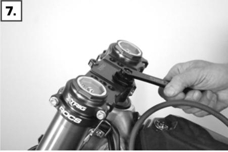
Screw the locking bolt (5) into the adjusting nut (4) and tighten with 10 Nm.
