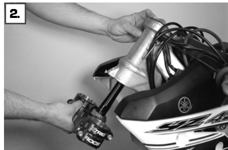
Slide the lower triple clamp into the steering head while holding the upper steering head bearing and sealing washer
