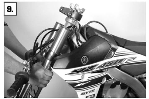
Pull out fork together with front wheel and brake system downwards
