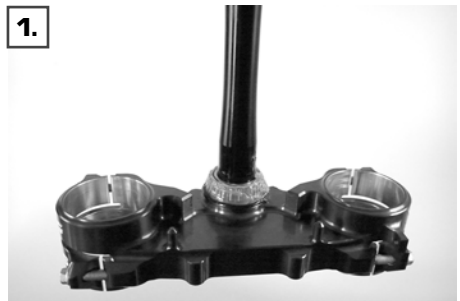
Grease the steering head bearing of the preassembled XTRIG triple clamp with suitable bearing grease
