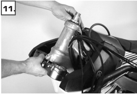
Hold the lower triple clamp and remove the adjusting nut of the steering head bearing
