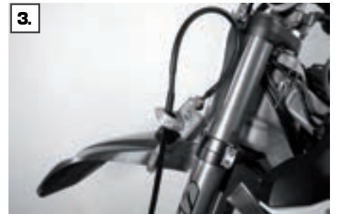
Mount brake pump on brake line
