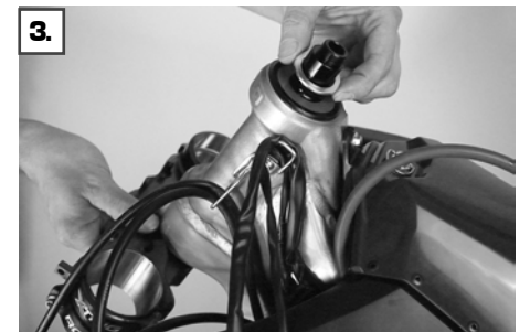
Depending on the model, install the seal for the steering head bearing (sealing ring or O-ring)
