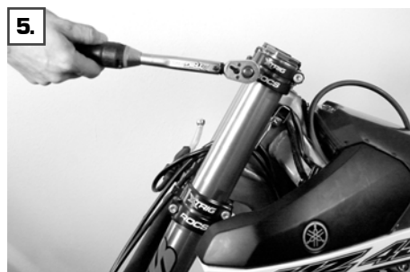
Insert fork including front wheel and brake system into the triple clamp
