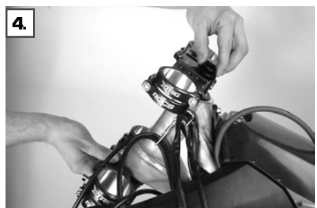
Place the upper triple clamp and tighten the adjusting nut (4) by hand
