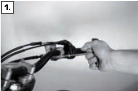
Dismantle brake pump
