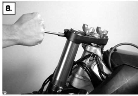
Loosen the clamps of the upper and lower triple clamp
