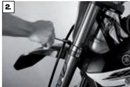
Dismantle brake line guide.
