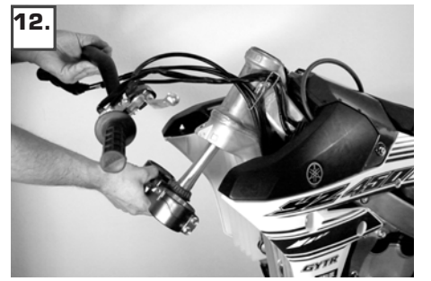
Dismantle the lower triple clamp. Clean the steering head and bearing seat of the motorcycle
