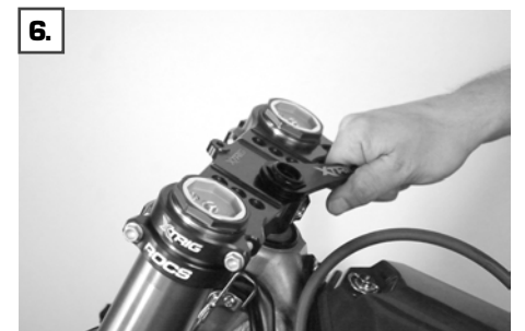
Set the required bearing clearance with the adjusting nut (4)
