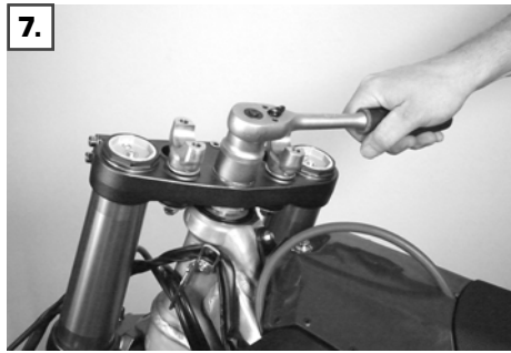
Loosen the fastening nut of the upper triple clamp
