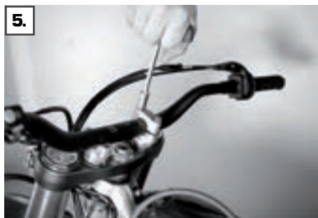
Dismantle handlebars and any fastening such as cable ties
