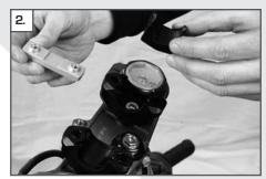
Insert the clamping bar (5) in the base support (1) (taper pointing up). Place the lower pan (6) in the clamping bar (5).
