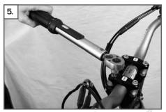
Evenly turn in the screws (10) and tighten to 16 Nm, making sure the clamping gap between the pans (6) + (7) is the same size (see photo correct/incorrect).
