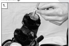
Screw (M10x25) (4) the base support (1) on the triple clamp with the pre-assembled tapered rubber (2) and tighten to 40 Nm. If necessary, add heighteners (3), using the M10x35 screws. NOTE: make sure you have the same offset direction.
